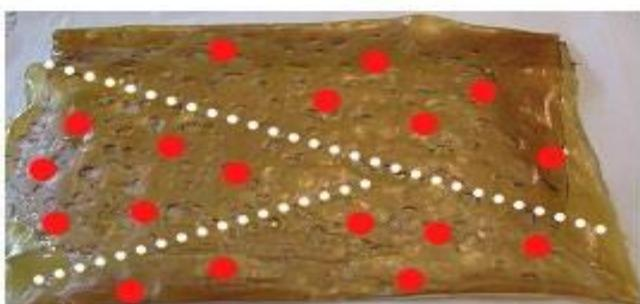
2. Determine the amount of sample increments from each section. Each sample increment should contain 0.5g of the product. Randomly collect same amount of sample increments from each thickness level. Sample increments shall be collected in a spacial pattern as indicated in "●".
